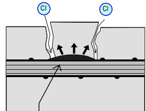
A crack arises to concrete with the expansion pressure of rust!!! Furthermore a steel rod becomes easy to rust.
