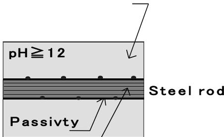
A steel rod is protected by passivity and does not rust.
