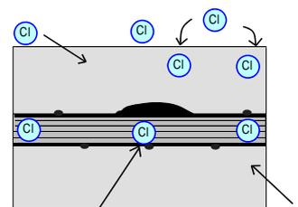
Chloride ion destroys passivity and a steel rod rusts. Chloride ion mixed together with sand etc.
