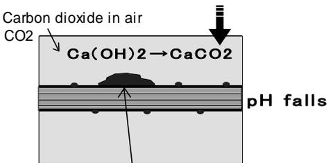
passivity of a steel rod is destroyed and it rusts.
