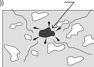
gelation absorbs and expansion swelling and a crack arises to concrete.
